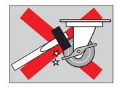
The design of the lock is required normal force to operate. Absolutely not apply grand force or it may damage the lock and parts.
