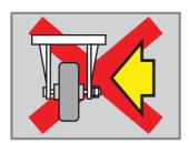
When operating the trolley with wheels fixed installation, you avoid horizontal forces impact on this type of wheel. If it's long-term impact or makes wheels turn, twist causing misalignment shorten the life of the product.
