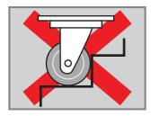
Do not push the car on the stairs, wheels are easy to be damaged by the impact of natural forces: vibration, inertial force when the cart "fall" from the top down to grade levels below.
