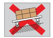
Firmly lock the cart when stopping or parking on ramp. Also need to put additional warning signs for people around the car may be gone downhill.
